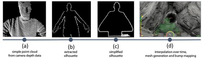
Fig. 3. Steps of the generation of the tunnel out of the Kinect stream
